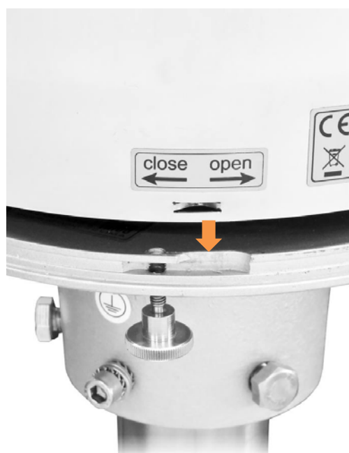
Figure 5: Re-assembly of the device
